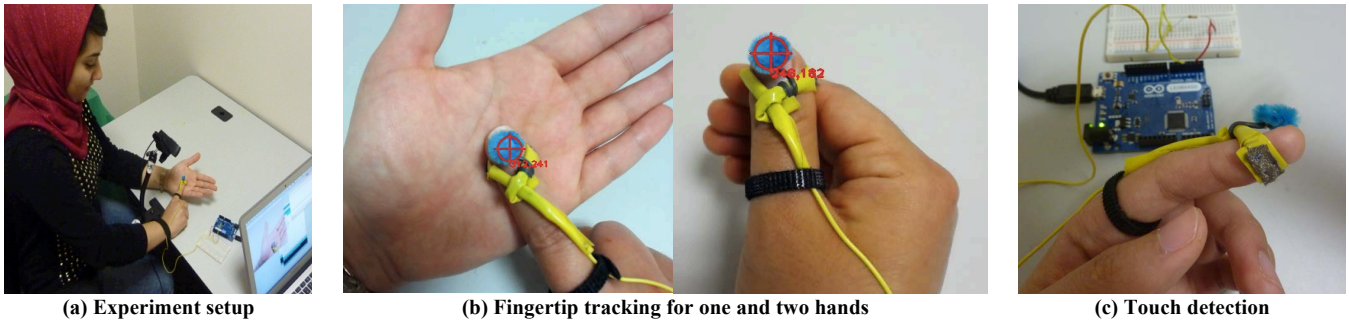
Figure 2. On-hand sensing system used in Task 2. Participants wore a lightweight ring that included a color marker (tracked by a camera) and a capacitive touch sensor. The ring could be placed so as not to cover the fingertip.
