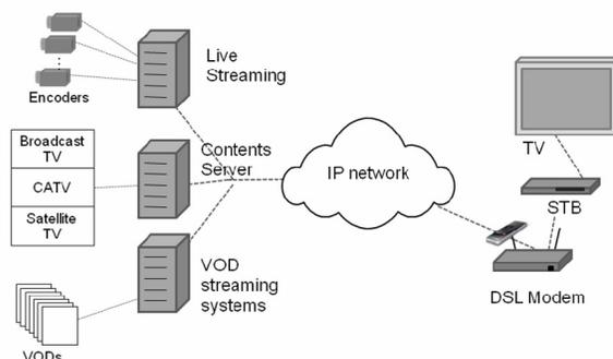
**Fig. 1. Architecture of an Internet Protocol Television (IPTV).** An IPTV set-top box (STB) is linked to a digital subscriber line (DSL) modem, and TV contents are delivered through the Internet Protocol (IP) networks.
