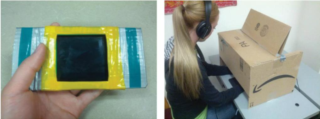
Fig. 1. Study 1 setup. (Left) Since the Samsung Galaxy Nexus screen has no tactile edge, we used a physical overlay to demarcate the active screen area. (Right) To impose eyes-free use, participants placed their hands inside of a box during tasks.
